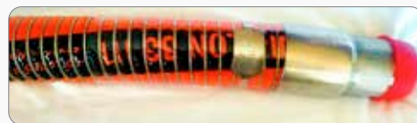
Clear heat shrink installed as a stress reliever
